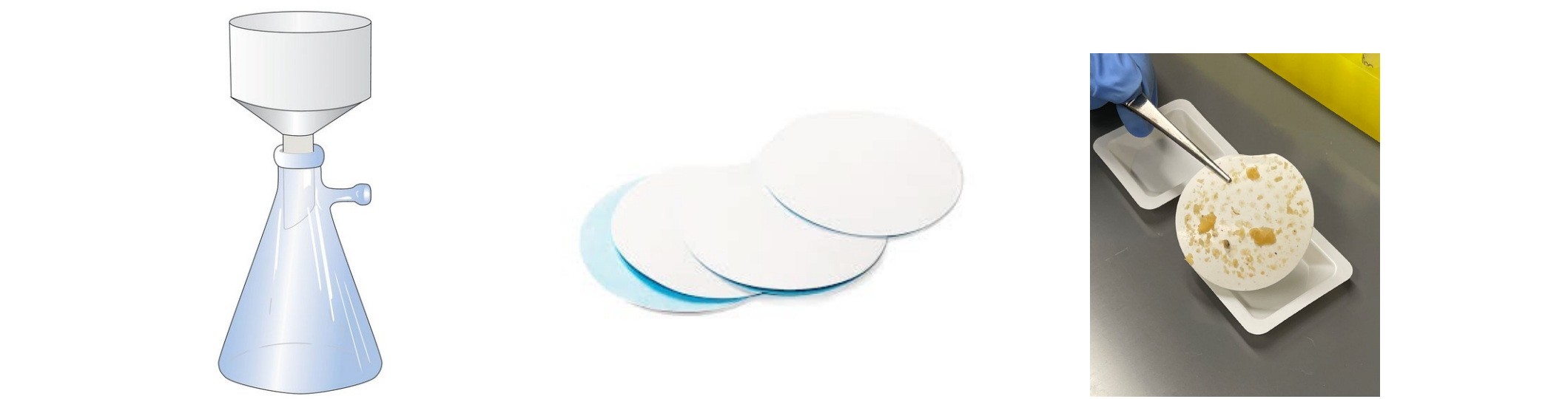
Fig. 4. Buchner Funnel diagram, nitrocellulose paper, and an example of filter paper after the water samples were filtered through.
